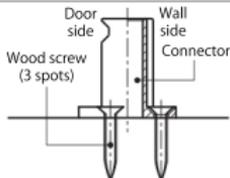
Please screw fixing screw with a phillips screwdriver.
